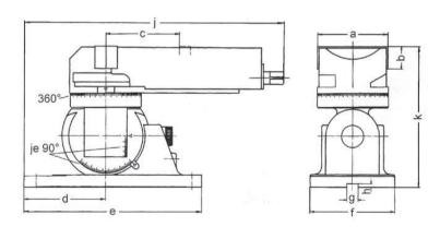
Clamping force: max. 20 kN at approx. tightening torque 60 Nm
